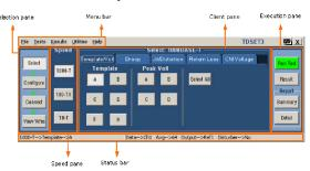
Click the Configure button from the Selection pane, or select Tests > Configure from the menu bar to change the configuration settings.
